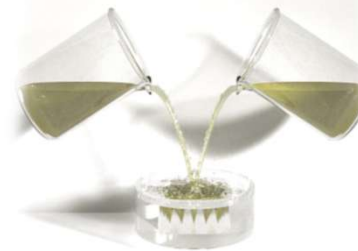
Silicone elastomers mixed and dried atop the master template
